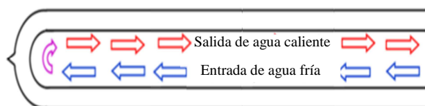
Figura 3: Tecnología del sistema water-in-glass
